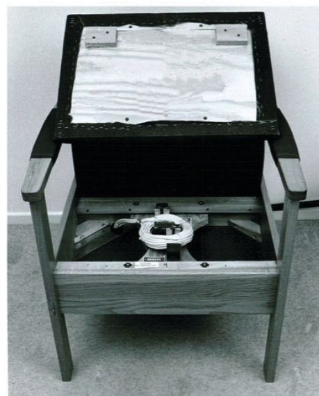
Figure 6 a-b. Magnetic chair showing magnetic field generator and external power unit (courtesy of Prof Kate Moore and Dr Alastair Morris, Sydney)
