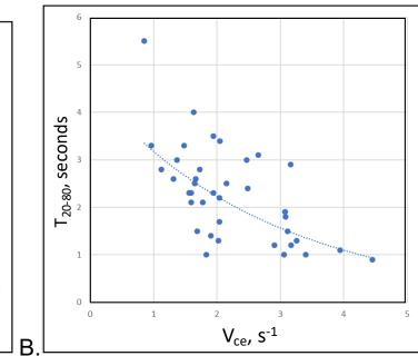
A. An example of the curve fitting of pressure data to obtain  $v_{CE}$ . The constant in the curve fit, used as an approximation to  $v_{CE}$ , is 1.78. The fit is acceptable, as  $R^2 > 0.4$ B. Correlation of  $t_{20-80}$  (DCP) with  $v_{CE}$  using data curves with  $R^2$  values greater than 0.4, suggesting that  $t_{20-80}$  values of greater than 2 seconds are found in the majority of poorly contracting detrusors. The R<sup>2</sup> value for the trend curve is 0.41.
