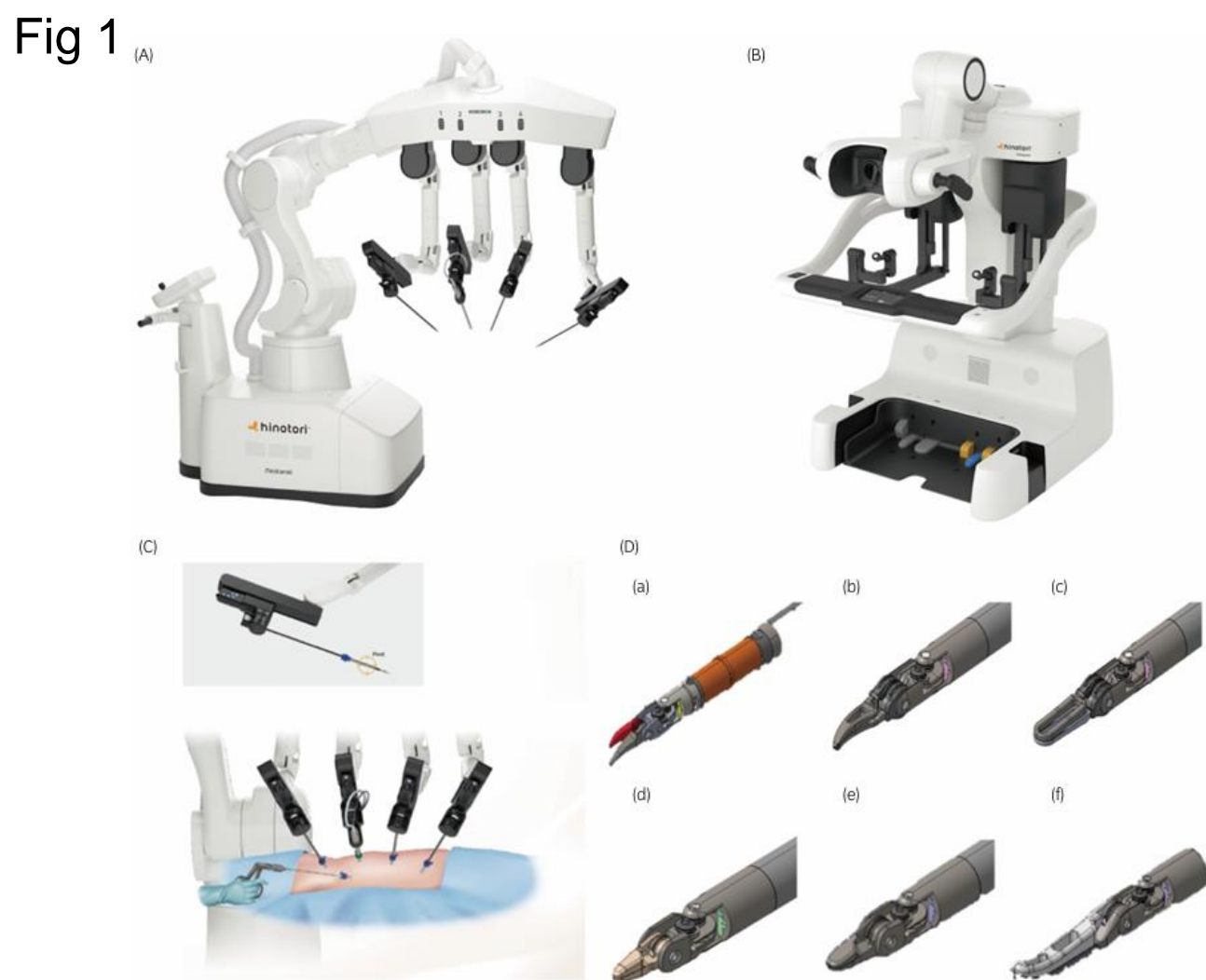
(A) Patient cart (B) surgeon's cockpit (C) docking-free design (D) instruments : (a) monopolar curved scissors, (b) bipolar Maryland forceps, (c) bipolar fenestrated forceps, (d) needle holder, (e) wide needle holder (f) Croce grasping forceps
